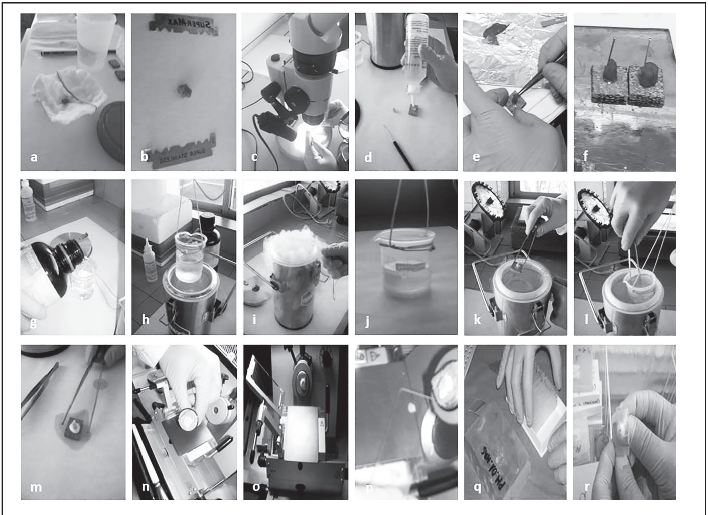
Figure 4. (a-f) Sequence of the procedure for mounting specimens for freezing. (b-l) Sequence of the procedure for freezing in isopentane cooled in liquid nitrogen. (m-r) Sequence for sectioning in cryostat and storage of slides and specimens.
